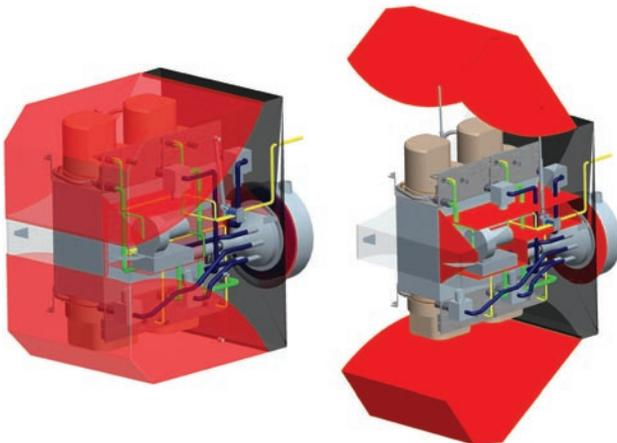
**FIGURE 5.** Latest SOFC APU Packaging and Integration
