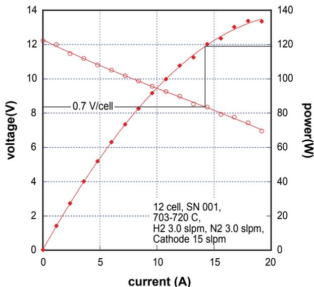
**FIGURE 2.** Polarization Plot and Power for 12-Scale Bundle
