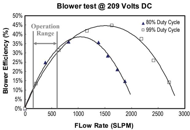
**FIGURE 4.** Flow vs. Efficiency for Cathode Air Blower (Operation Range: 136 to 570 SLPM)
