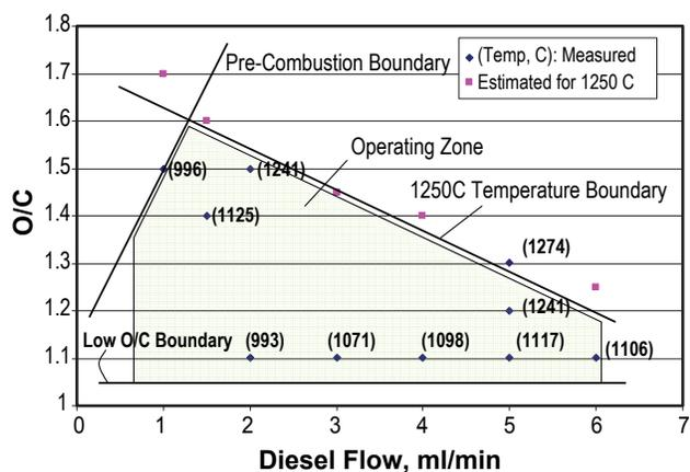
**FIGURE 1.** O/C vs flow rate which determines the estimated operating window for the B2 catalyst at a feed preheat temperature of about 325°C.
