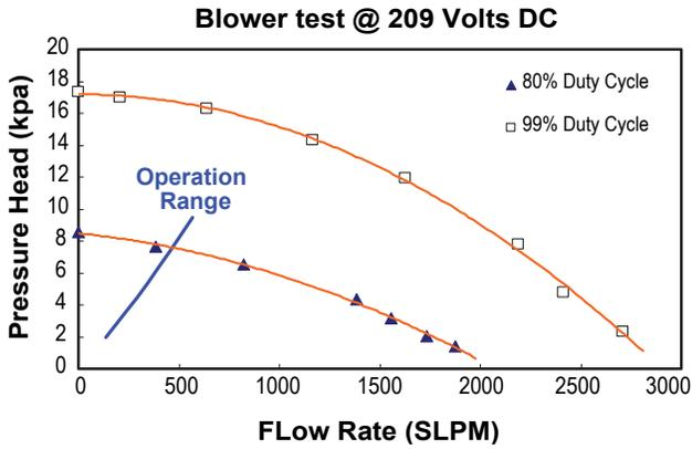
**FIGURE 3.** Flow vs. Pressure Head for Cathode Air Blower (Operation Range: 136 to 570 SLPM)
