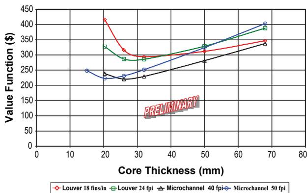
FIGURE 3. Curves Represent the Value Function Vs. the Radiator Thickness for Four Fin Configurations
