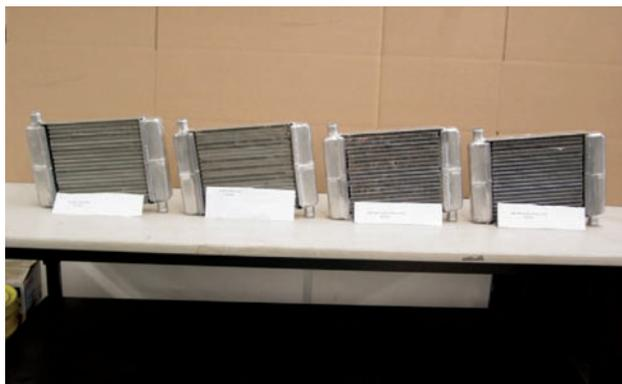
FIGURE 4. Sub-Scale (9" x 9") Radiators with Four Different Fin Configurations
