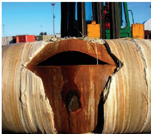
FIGURE 1. Burst Test of Composite Over-Wrapped Steel-Lined Pressure Vessel
