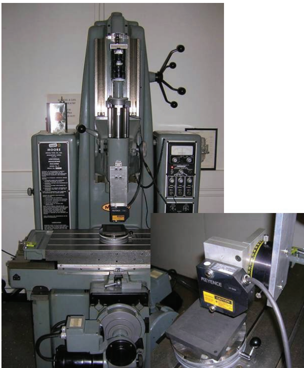
FIGURE 4. Phase 2 Testing: 3-Axis Machine Tool with Probe 1 Mounted to Machine’s Z-Axis
