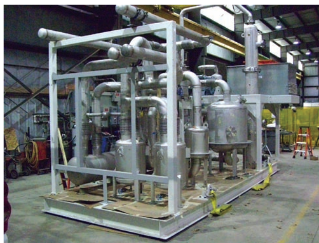
FIGURE 4. Anode Exhaust Skid Fabrication
