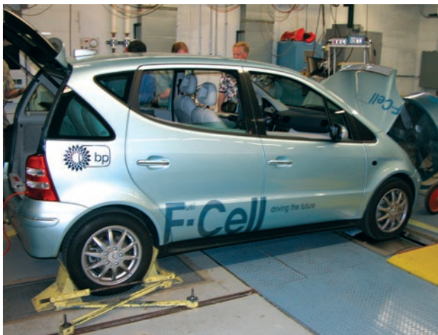
FIGURE 2. Gen-I Dynamometer Testing
