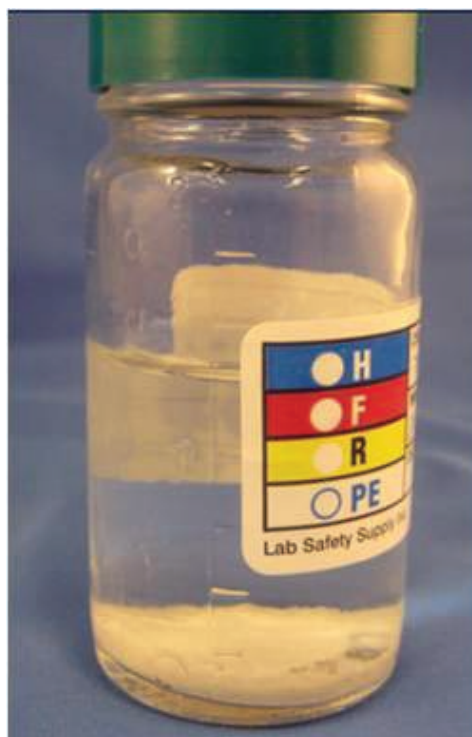
FIGURE 2. Reaction product liquor from hydrolysis and liquid phase reforming of 1 wt% yellow poplar at 310°C in 0.1M K 2 CO 3 with a 0.5 L/min N 2 sweep gas. White sediment is potassium titanate, a titanium corrosion product.
