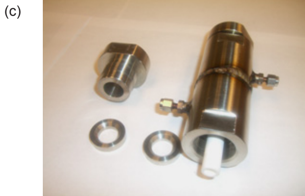
FIGURE 5. (a) Schematic of membrane reactor setup for WGS reaction, (b) CO conversion for WGS reaction under H_2O/CO ratio of 1 and space velocity of 3,500\text{ h}^{-1} in the disk-shaped silicalite membrane reactor with Fe/Cr WGS catalyst, fixed-bed reactor, (c) Tubular WGS membrane reactor.
