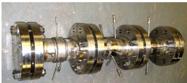
FIGURE 1. Three-Module Integrated WGS/Membrane Device
