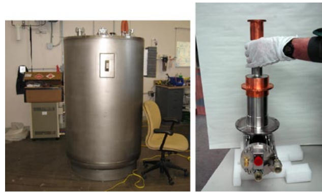
FIGURE 4. The AMRL cold box on the left is a double-walled Dewar. The cryocooler on the right is a proven two-stage Gifford McMahon model used for conduction cooling of the magnet and thermal shield.
