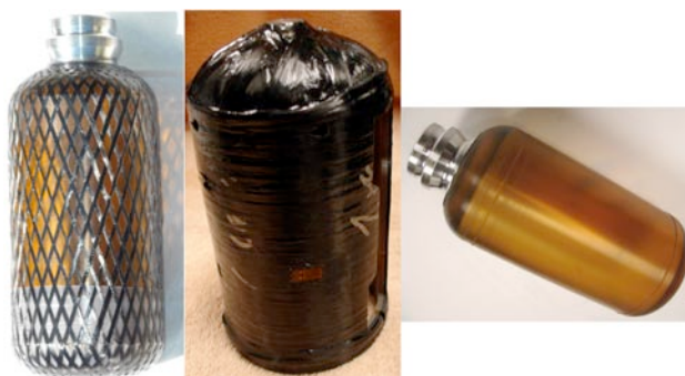
FIGURE 1. Photographs of early test articles built and destroyed to test new matrix and liner plastic formulations and manufacturing processes. Dozens of 3" subscale pressure vessels have been built and burst tested. The figure shows a liner test article with partial graphite overwrap intended to test liner burst strength (left), a sectioned fully overwrapped vessel designed to burst at 3,000 psi with dog bone tensile test specimens cut from as-built walls (center), and a liner with 3,000-psi boss design ready for overwrapping (right).
