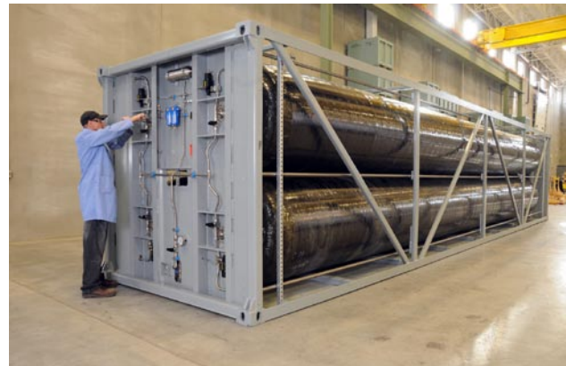
FIGURE 3. Final Assembly of TITAN ISO Frame System
