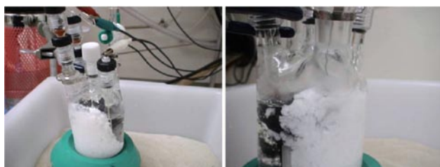
FIGURE 4. TEDA is known to complex with \text{AlH}_3 , appearance of precipitate signals alane molecule formation.
