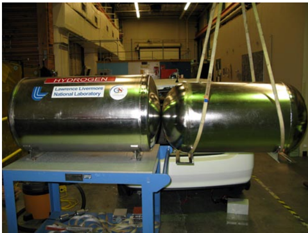
FIGURE 1. Generation 2 (left) and generation 3 (right) cryogenic pressure vessels. Generation 3 vessel is 23% more compact through reduced insulation thickness (1.5 cm vs. 3 cm).
