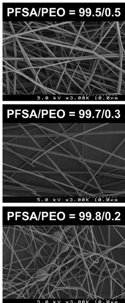
FIGURE 1. SEM surface images of nanofiber mats, made by cospinning 825 EW PFSA (from 3M Corp.) with 10 6 MW PEO (3,000x magnification). The PFSA/PEO weight ratio in the spinning solution is listed above each micrograph.
