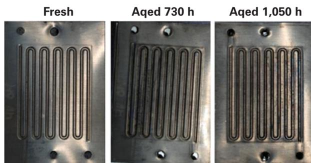
**FIGURE 3.** Macrographs of cathode-side stamped and pre-oxidized/nitrided Fe-20Cr-4V test foils as-nitrided and after 730 and 1,050 h of single-cell fuel cell testing.
