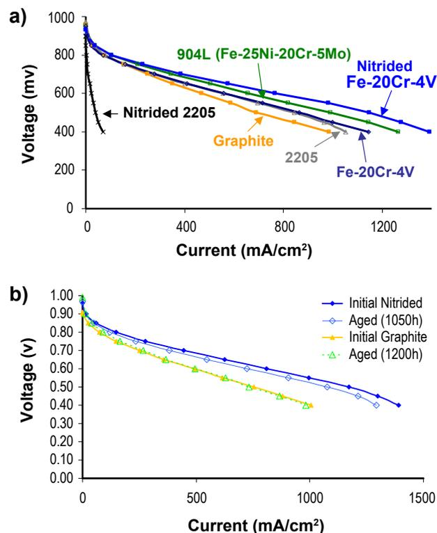
**FIGURE 2.** Single-Cell fuel cell test V-I curves. a) initial performance; b) performance of 1,000<sup>+</sup> h aged plates using a fresh MEA.
