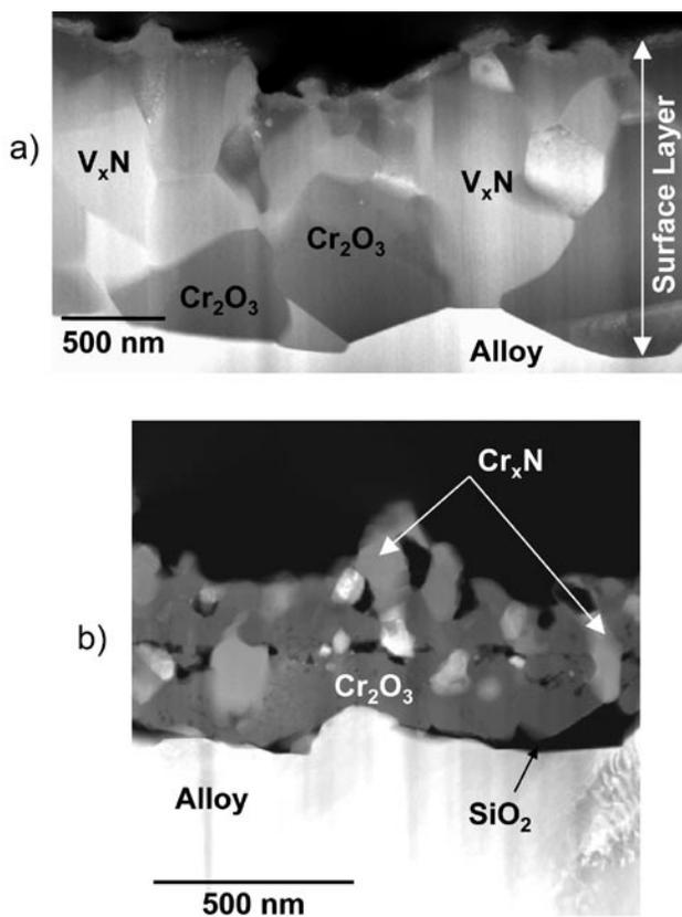
**FIGURE 1.** High angle annular dark field scanning transmission electron microscopy cross-section of pre-oxidized and nitrided Fe-20Cr-4V (a) and 2205 (b) stainless steel foils.
