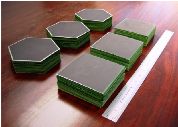
FIGURE 1. Picture of 360 Cells to be Assembled into Six Modules
