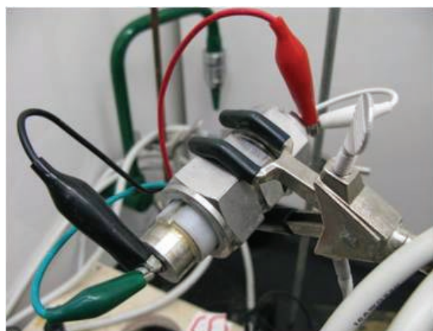
FIGURE 3. Swagelok Cell Connected to a Potentiostat for Cycling
