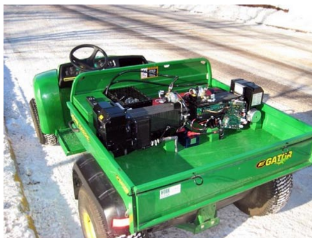
FIGURE 1. John Deere e-Gator with Hydrogen Power Plant In Vehicle Bed
