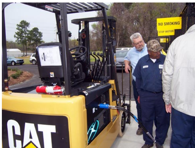
FIGURE 1. LiftOne Truck Fueling at the Columbia, SC, Hydrogen Station
