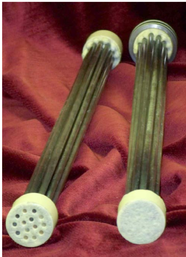
FIGURE 4. Photo of the standard 2 nd generation Pd (i.e., candle filter) bundle showing the open and closed ends.
