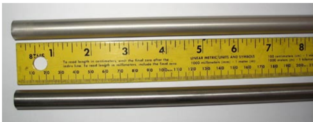
FIGURE 2. Surface of tubular membrane before and after catalyst deposition. An as-received tube is shown on the bottom and a tube with deposited catalyst is shown on the top.
