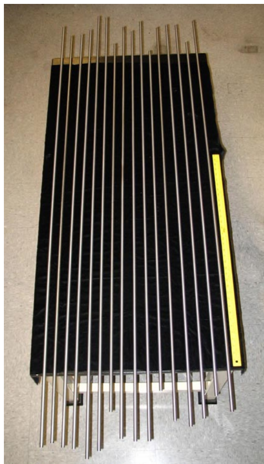
FIGURE 1. Digital image of as-received tubular membranes. A yardstick is included on the right side of the picture for reference.
