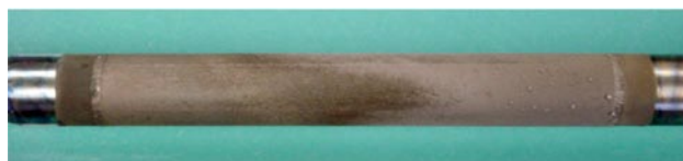
FIGURE 3. The used Sn/Inconel Membrane after Permeation Experiments up to 600°C
