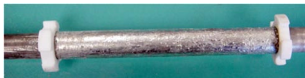
FIGURE 2. A 20 \mu m Dense Layer of Sn on the Porous Inconel Support before Permeability Test
