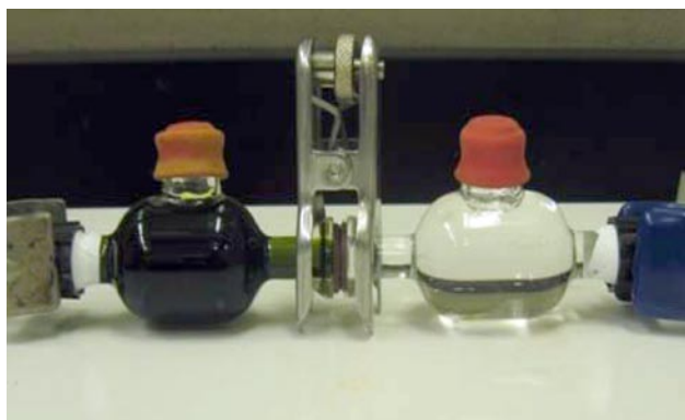
FIGURE 1. Diffusion cell set up for testing membrane with a solution of \text{CuCl}_2 in 10.2 M HCl solution on the solute-rich side and 10.2 M HCl solution on the solvent-rich side.
