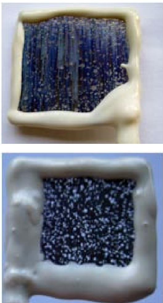
FIGURE 2. Top, an uncoated hybrid photoelectrode after -3 \text{ mA/cm}^2 was applied in \text{pH}_2 buffer for 24 hours. The image on the bottom is of a different hybrid photoelectrode subjected to the same conditions after 48 hours.
