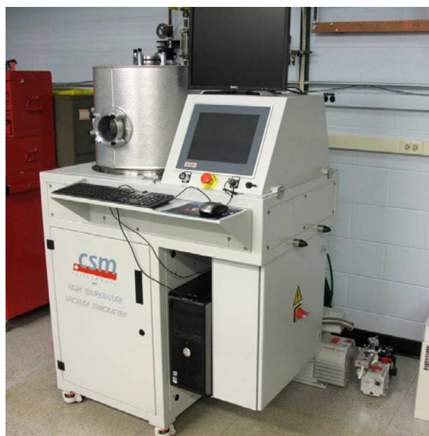
FIGURE 1. Photograph of New High-Temperature Hydrogen Test Machine
