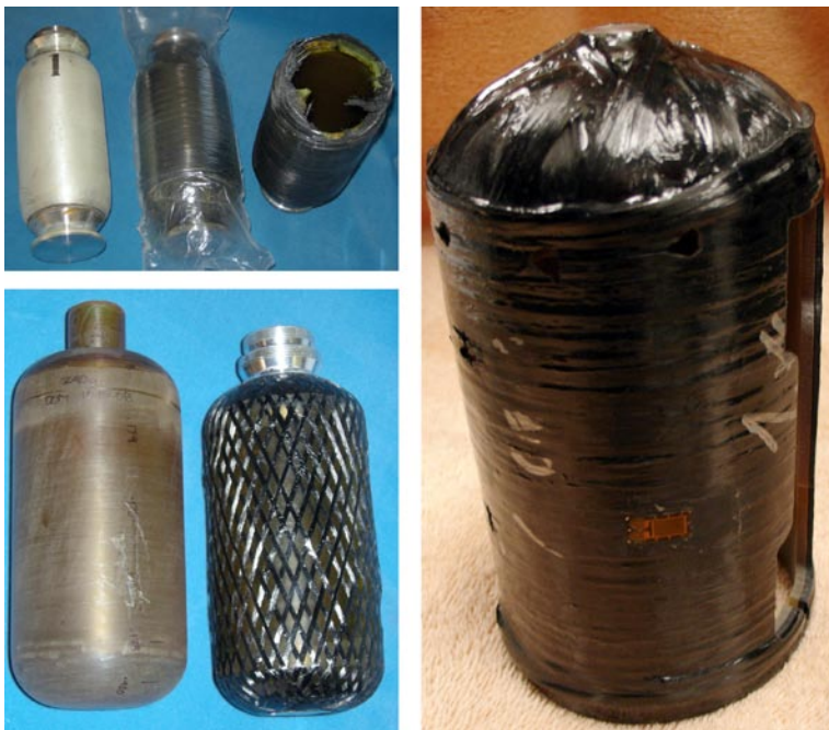
FIGURE 1. Subscale Pressure Vessels: 3" diameter tests articles photographed in a number of experimental configurations. In the photograph at top left, a metal-coated, glass composite vessel is shown at left with stainless steel bosses configured for permeation tests, next to a bagged advanced plastic composite matrix vessel, and a view into the blown out bottom of a failed vessel. In the photograph at lower left, a liner spin cast from advanced plastic awaiting filament winding and boss installation at its top end appears next to an attempt to use these 3" articles to test the strength of the liner only, inside a partial-coverage winding of graphite epoxy composite. The photograph at right shows the bottom of a sectioned, completed, and tested to failure vessel which has been sliced to examine failure in its boss-side dome form from the inside, after "dog bone" tensile test specimens have been cut out of its side with a water jet.
