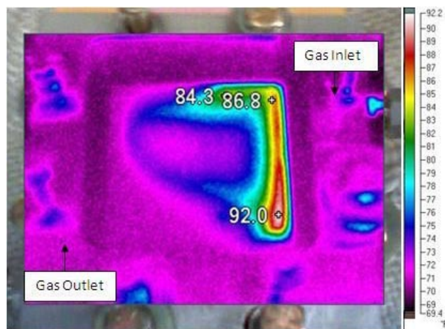
FIGURE 2. Infrared image of the hot spots on an MEA from a tested fuel cell. Hot spots are noted with approximate temperatures based on the emissivity of carbon.
