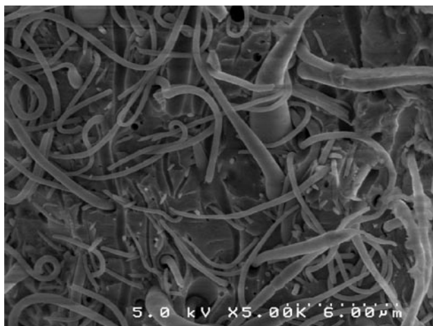
FIGURE 1. Freeze-fractured SEM cross-section of a Nafion®/PPSU nanofiber composite membrane (with Nafion® surrounding PPSU nanofibers; 70 vol% Nafion®).
