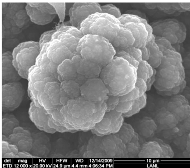
FIGURE 1. Typical dendrite structure of a polypyrrole film electrochemically deposited onto a glassy carbon electrode in absence of any template molecules.
