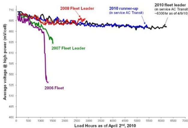
FIGURE 1. Comparison of Performance Loss at High Power for Various Generations of PM120 Bus Power Plants
