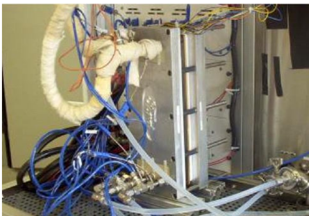
FIGURE 4. Picture of the 10-cell Short Stack under Long-term Stability Test at Ford
