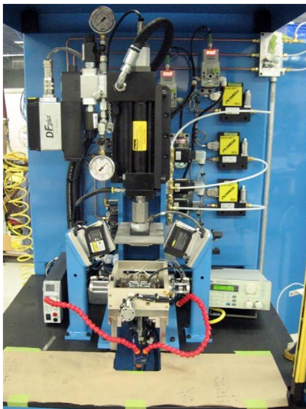
FIGURE 2. Leak-Test Suite Prototype: Test Fixture
