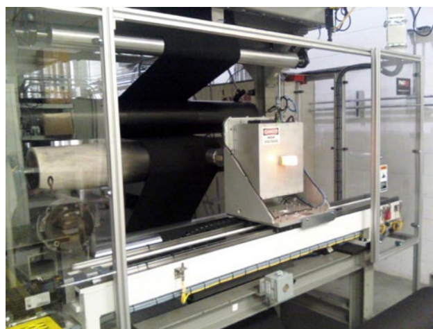
FIGURE 1. Picture of Custom-Designed In-Line Analyzer for Precious Metal on Gas Diffusion Electrodes
