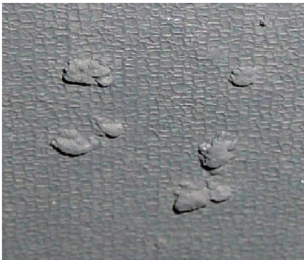
FIGURE 2. Example of Agglomerates Found on Gas Diffusion Electrodes
