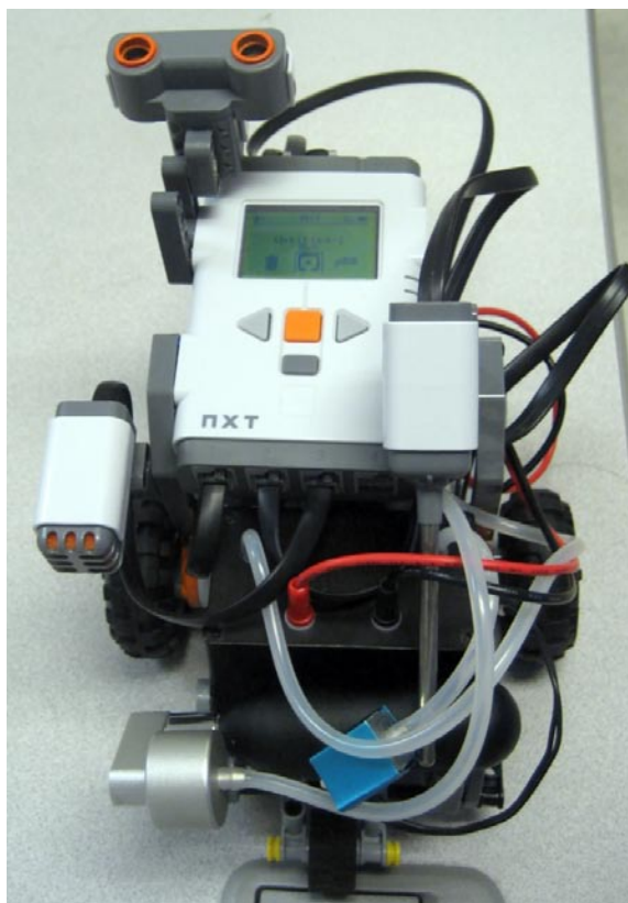
FIGURE 2. The very first in the world LEGO Mindstorm robot powered by a 20 W Horizon fuel cell.
