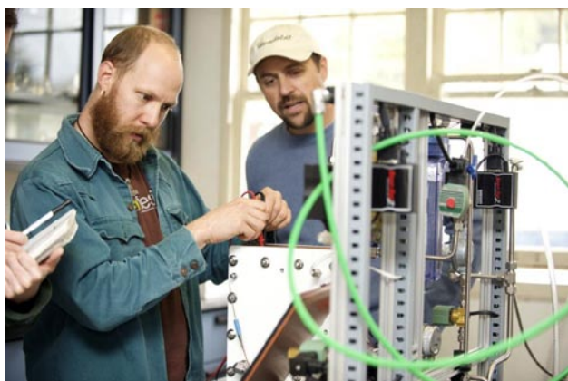
FIGURE 2. HSU engineering student measures fuel cell voltages on H_2E^3 test station while SERC fuel cell engineer Greg Chapman looks on.
