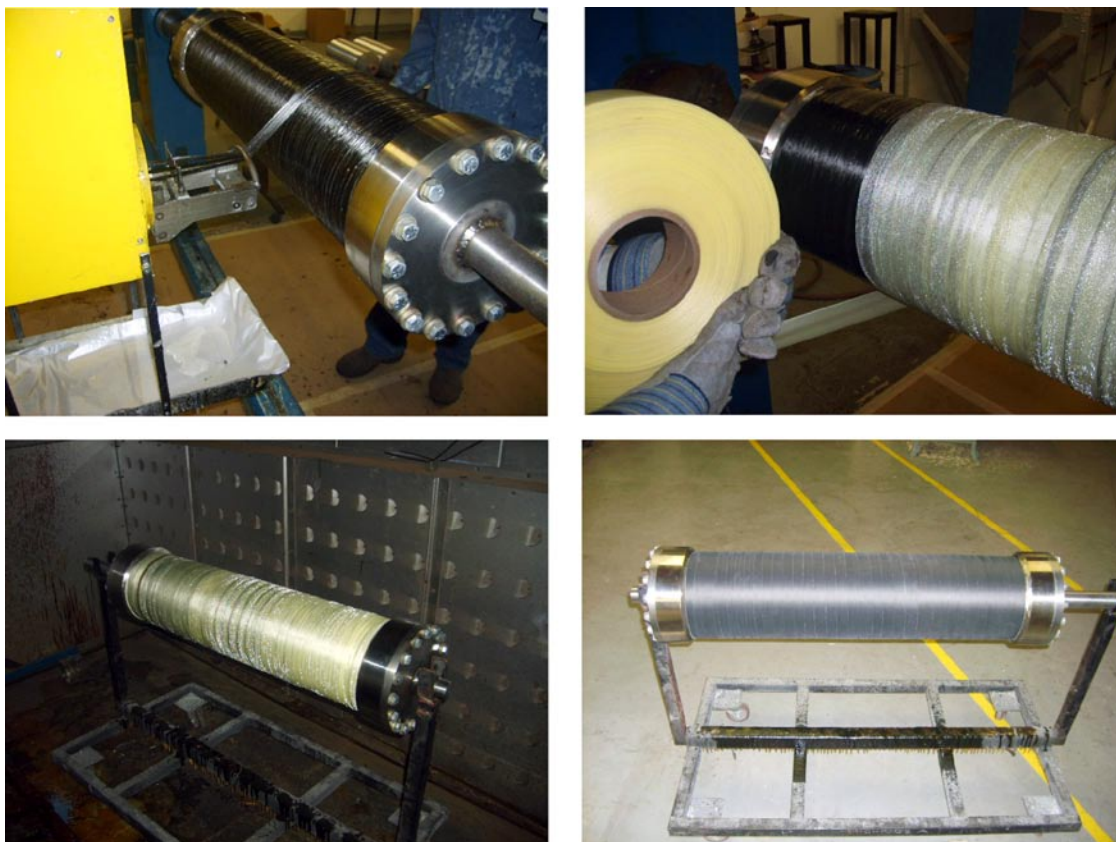
FIGURE 4. HyperComp Wrapping Sequence and Finished Cylinder
