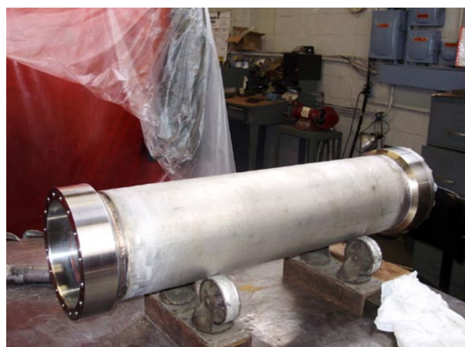
FIGURE 3. Photograph of Cell Prior to Carbon Fiber Wrapping
