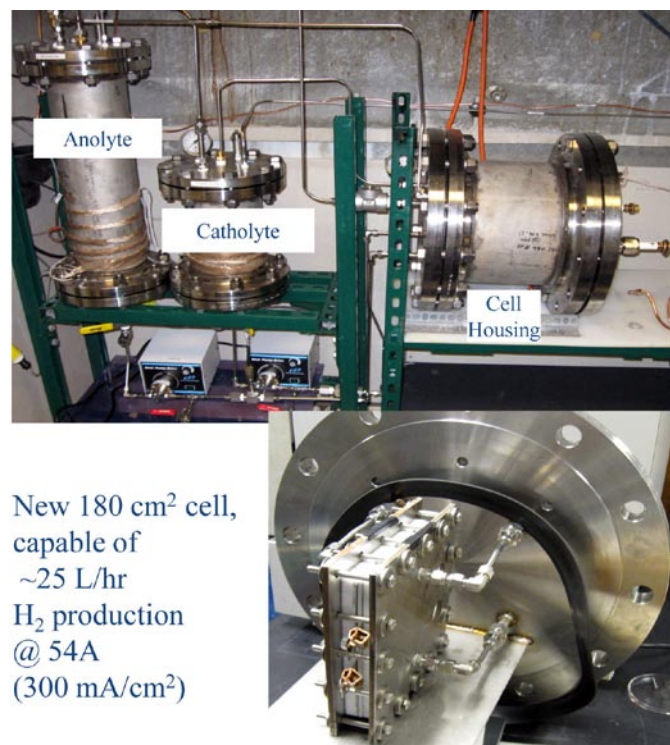
FIGURE 3. Pressure Vessels Required for Electrochemical Cell Operation at High Temperature
