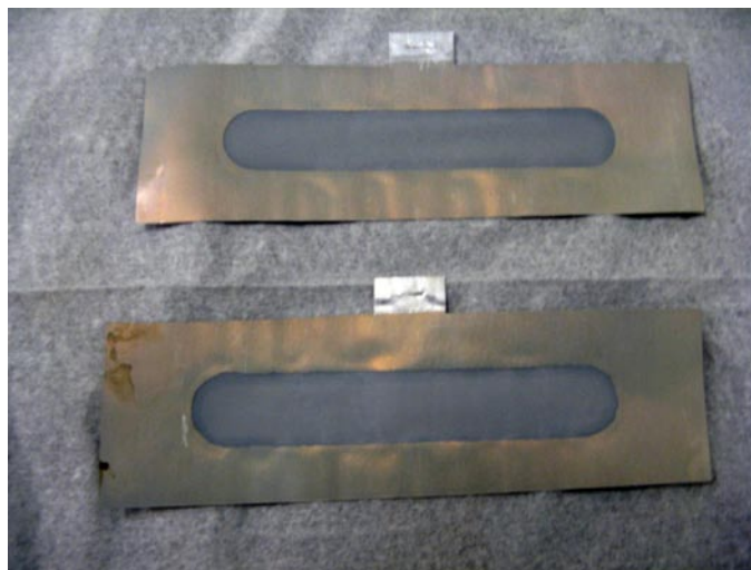
FIGURE 1. Annealed 1"×5" AAO Membranes Supported by Aluminum Rim
