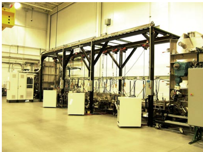
FIGURE 1. Xunlight's Roll-To-Roll Deposition System For Large-Area Fabrication of PEC Electrodes
