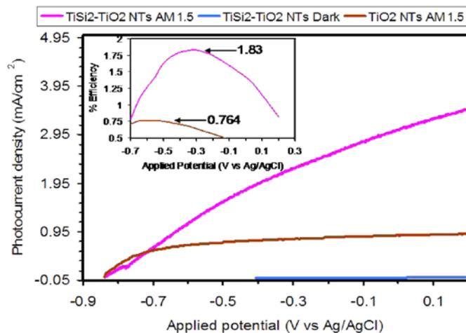
**FIGURE 7.** Potentiodynamic plot of annealed  $\text{TiSi}_2/\text{TiO}_2$  NTs and  $\text{TiO}_2$  NTs. Inset shows the solar-to-hydrogen conversion efficiency of  $\text{TiSi}_2/\text{TiO}_2$  NTs and  $\text{TiO}_2$  NTs under AM 1.5 illumination.
