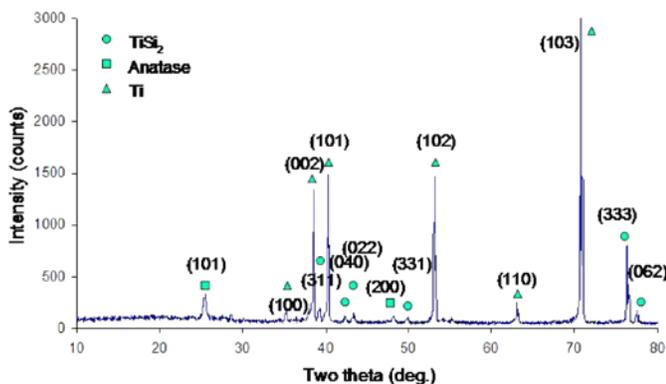
**FIGURE 5.** Glancing angle X-ray diffraction pattern of  $\text{TiSi}_2$  NP/ $\text{TiO}_2$  NT. Orthorhombic  $\text{TiSi}_2$  and anatase  $\text{TiO}_2$  are observed in the heterostructure. A peak for the Ti base is also noticed.
