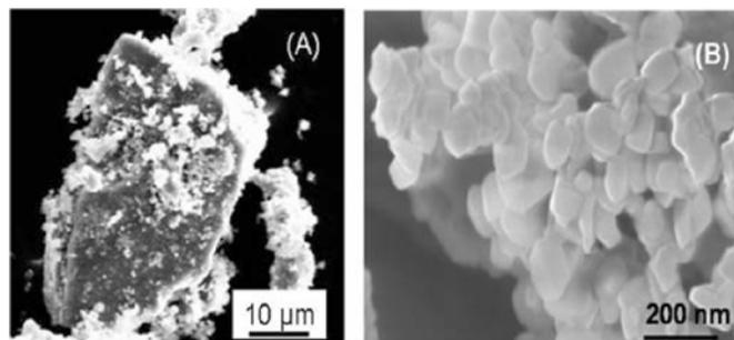
**FIGURE 3.** Field emission scanning electron microscope images of (A) as-received  $\text{TiSi}_2$  particles ( $<44 \mu\text{m}$ ), (B) ball-milled  $\text{TiSi}_2$  particles ( $\sim 50\text{-}60 \text{ nm}$ ).
