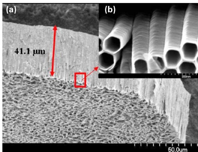
**FIGURE 2.** Field emission scanning electron microscope images of  $\text{TiO}_2$  NTs prepared in organic medium at  $80 \text{ V}_{\text{DC}}$  for 30 min. (a) top view and (b) cross sectional view (close-up) view of the NTs.
