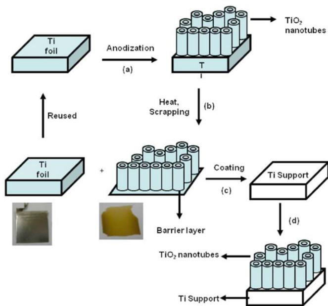
**FIGURE 1.** Schematic Showing the Formation of  $\text{TiSi}_2/\text{TiO}_2$  NT Composite Structure
