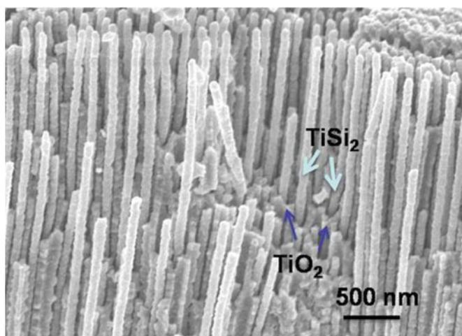
**FIGURE 4.** Field emission scanning electron microscope images of  $\text{TiSi}_2$  particles sintered into the  $\text{TiO}_2$  NT array.
