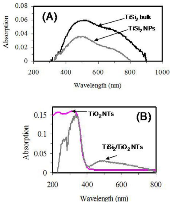
**FIGURE 6.** Diffuse reflectance ultraviolet and visible spectra of (A)  $\text{TiSi}_2$  bulk and nanoparticles and (B)  $\text{TiO}_2$  NTs and  $\text{TiSi}_2/\text{TiO}_2$  NTs catalyst.  $\text{TiSi}_2$  particles showed absorption in the visible light region and  $\text{TiSi}_2/\text{TiO}_2$  NTs absorb light in both ultraviolet and visible region. Band gap =  $2.25$  eV.
