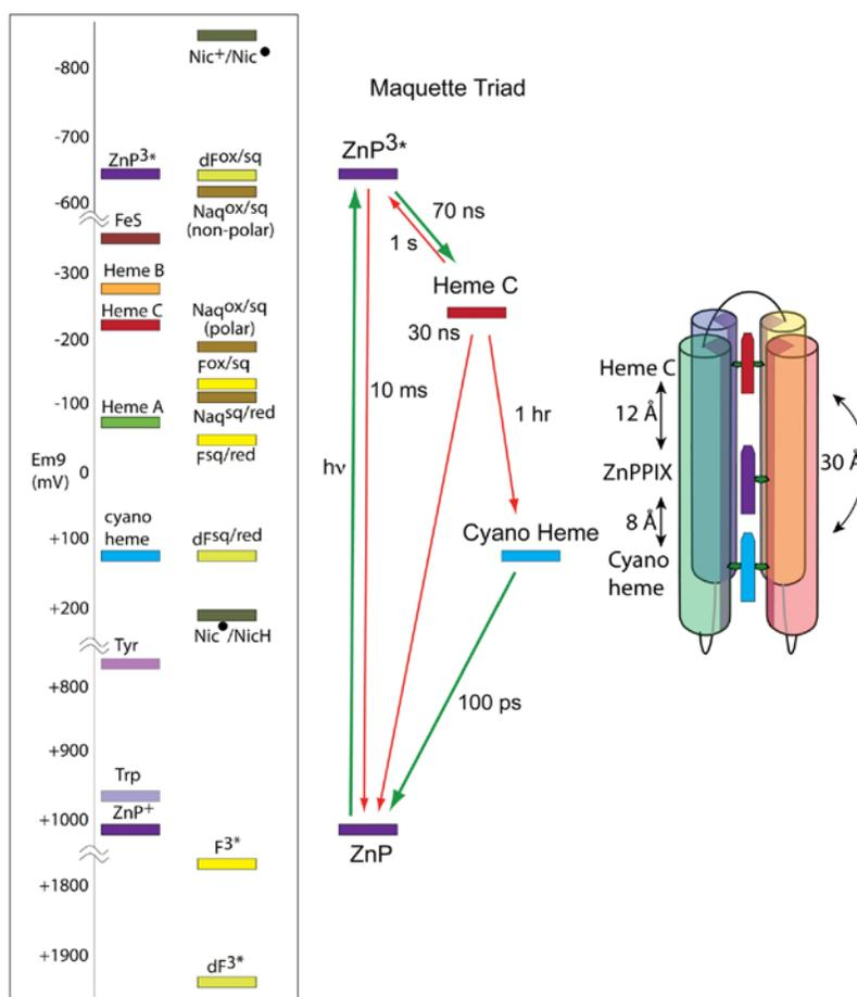
Average energy levels of redox centers secured inside maquettes. The first column on the left lists one-electron donors/acceptors and the second column two-electron cofactors. The middle schematic shows energy levels and lifetime selected in a triad presently under construction depicted on the right.
