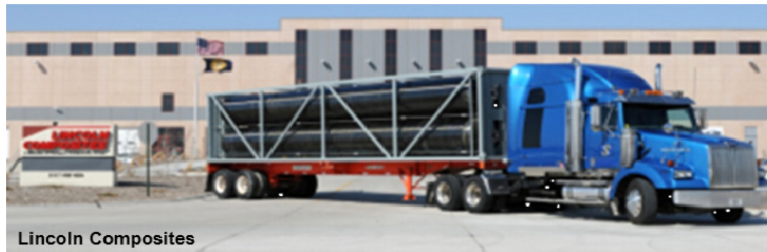
FIGURE 2. Carbon Fiber Composite Tube Trailer Pressure Vessel and International Standards Organization Container
