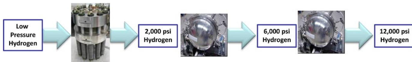
FIGURE 3. Multi-Stage System Capable of Reaching 12,000 PSI
