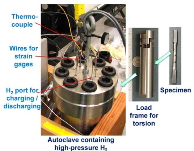
**FIGURE 1.** Special, in situ testing apparatus for measuring fracture toughness degradation of materials exposed to high-pressure hydrogen
