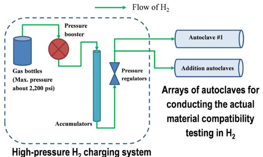
**FIGURE 4.** Schematic of a hydrogen charging system capable of maintaining or varying pressure up to 10,000 psi
