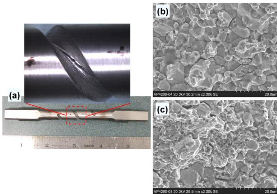
**FIGURE 2.** (a) Surface appearance of a fractured sample after hydrogen exposure, (b) SEM image of fracture surface near the notch root, and (c) SEM image of fracture surface away from the notch root
