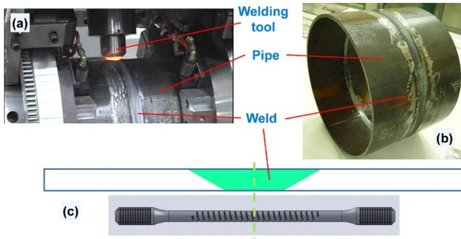
**FIGURE 3.** (a) Snapshot of FSW of X-65 steel pipe sections, (b) resulting pipe girth weld, and (c) schematic drawing of multi-notch tensile specimen
