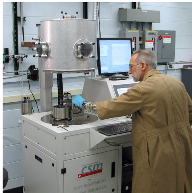
FIGURE 1. Photograph of new high-temperature hydrogen test machine in open position for loading of test specimens.
