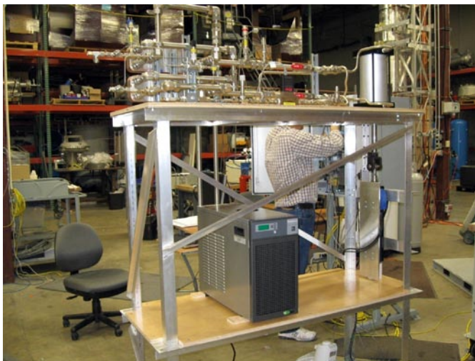
FIGURE 6. Heat Transfer Fluid Subsystem Components
