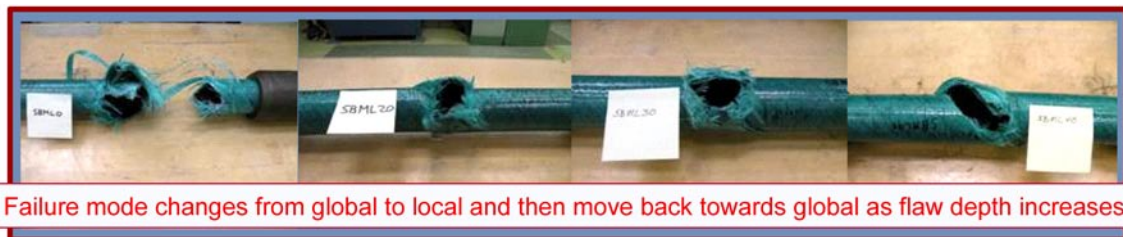
FIGURE 3. Photo Illustrating Failure Mode of FRP
