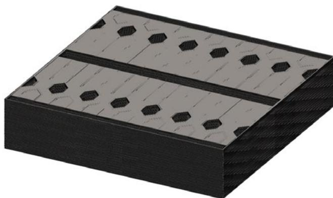
**FIGURE 4.** Schematic Diagram of  $\mu$ CHX
