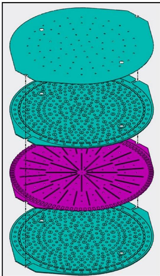
**FIGURE 2.** Schematic Diagram of Cooling plate including One Hydrogen Distribution Lamina (Purple) and Two Cooling Fluid Lamina (Teal)
