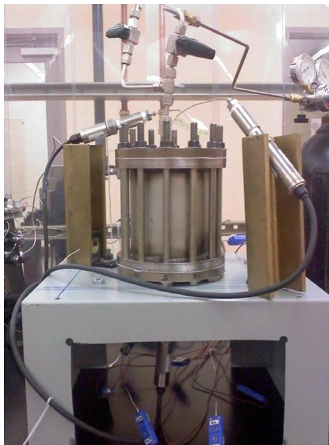
**FIGURE 3.** Modular Adsorption System Test Apparatus
