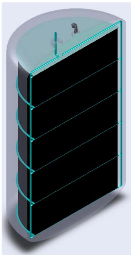
**FIGURE 1.** Schematic Diagram of Modular Adsorption System including Five Modules and Cooling Fluid Headers
