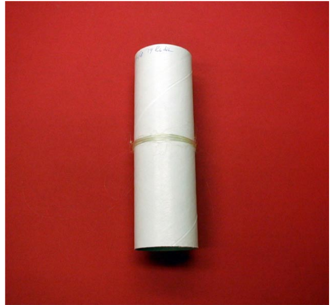
FIGURE 4. Melt-spun PAN/VA fibers using 19-filament die (0.0022" in diameter). The diameter of fibers is about 10 to 20 microns.
